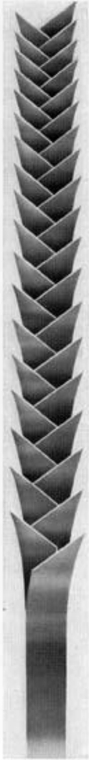
Looking down the cutting edge of a crosscutting Hand saw--as it appears in an enlarged view.
